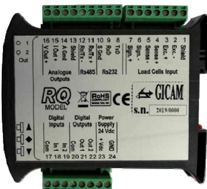
Depending on the version of the RQ ordered (RS485, Analog, Ethernet, Profibus, Profinet, CANopen, DeviceNet) not all connections are available. Connections not indicated above are made through special connectors (D-Sub etc.).
