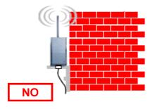
Do not install the instrument too close to walls. The ideal distance should be greater than 35 cm from the antenna.
